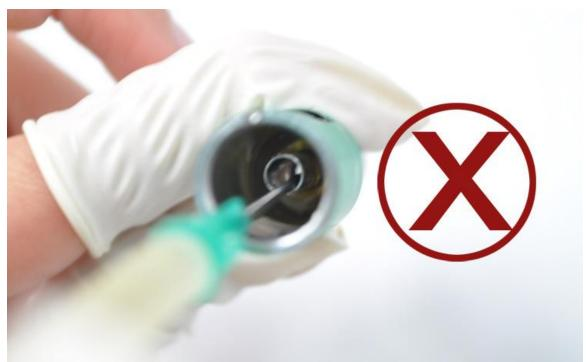
Do NOT fill down the centre tube. Also do not fill past the opening of the air centre tube as liquid will flow into the tube.
