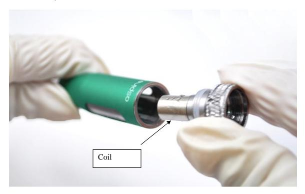
2. Unscrew the Coil from the base and replace with a new one. Replacement Coils can be purchased separately.
